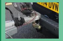
Disconnect the breakaway cable and stow away safely.
